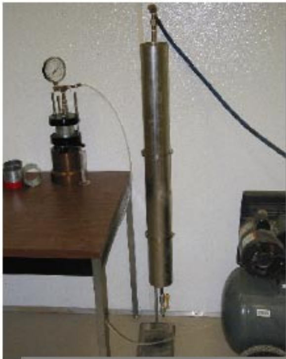
Figure 12. AFRL constant-head permeability test apparatus for concrete.
