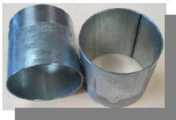
Figure 16. Sample molds for concrete permeability test.
