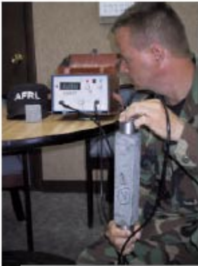
Figure 8. AFRL modulus of elasticity test performed by an AFRL/MLQD engineering aide.
