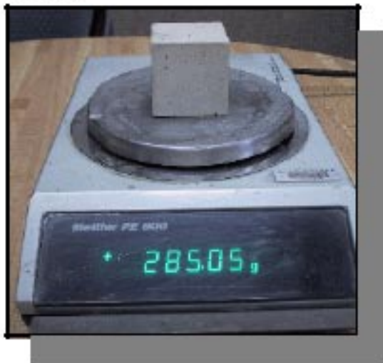
Figure 3. Density test setup for a sample of chemically-bonded fly ash.
