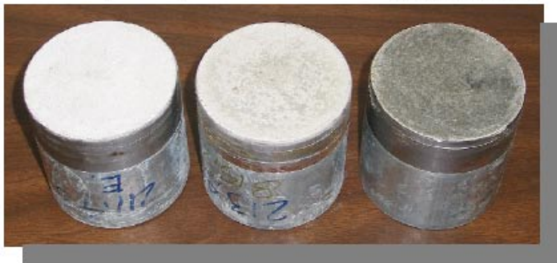
Figure 18. Concrete permeability test specimens, from left to right: (1) standard Portland cement mortar; (2) standard Portland cement mortar plus 10% raw fly ash (by dry weight); and (3) chemically-bonded fly ash.
