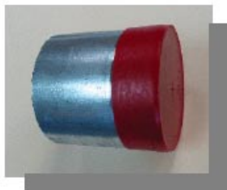
Figure 17. Sample mold with bottom cap installed.
